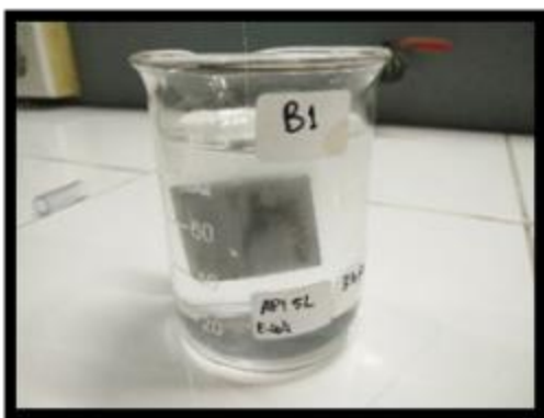
Figure 5 Immersion material on media bio-corrosion
