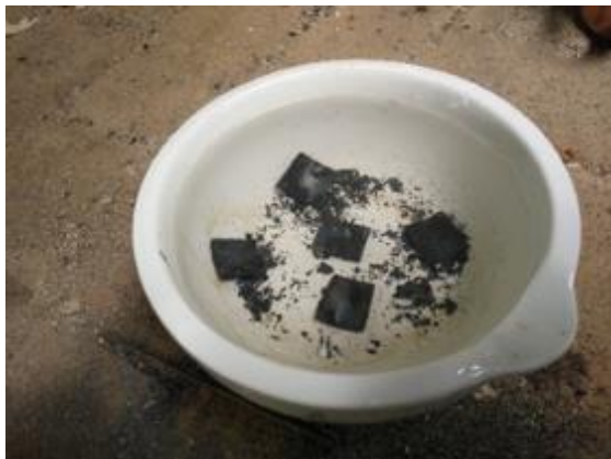
Figure 7. The process of rapid cooling water media
